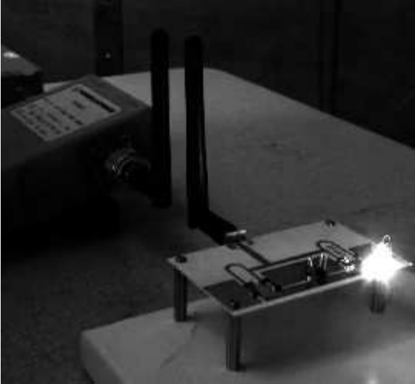
Fig. 10. Photograph of a string of four LEDs being wirelessly powered by the TLRCN/rectifier system.
