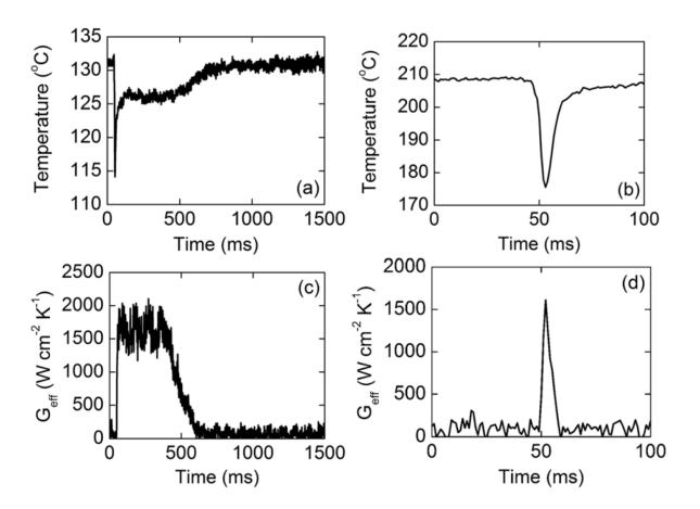
**Figure 9:** Illustrative data showing transient changes of temperature and effective thermal conductance created by the impingement of dispensed water volume of 0.19 mm<sup>3</sup>. Panels (a) and (c) are for a relatively low sample temperature of 130 °C. Panels (b) and (d) are for a relatively high sample temperature of 210 °C. Time zero is defined by the electronic trigger of the microdispenser. The series of water droplets arrives at the sample surface 50 ms after the trigger.
