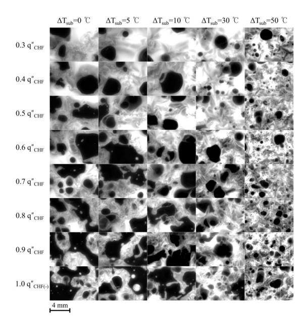
**Figure 3:** Phase distribution on the boiling surface at various values of heat flux (normalized to CHF) and subcoolings, obtained with eth DEPIcT technique. Black represents dry regions, grey and white represent wet regions. The fluid is water at atmospheric pressure, boiling over horizontal silicon heaters. Note that the subscript 'CHF(-)' indicates the last heat flux step before CHF occurs.
