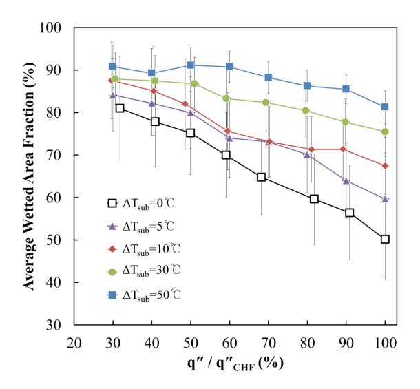
**Figure 4:** Post-processing of the DEPIcT data in Figure 5 yields the time-averaged wetted fraction (i.e. fraction of boiling surface that is contact with the liquid phase) as a function of normalized heat flux and subcooling.
