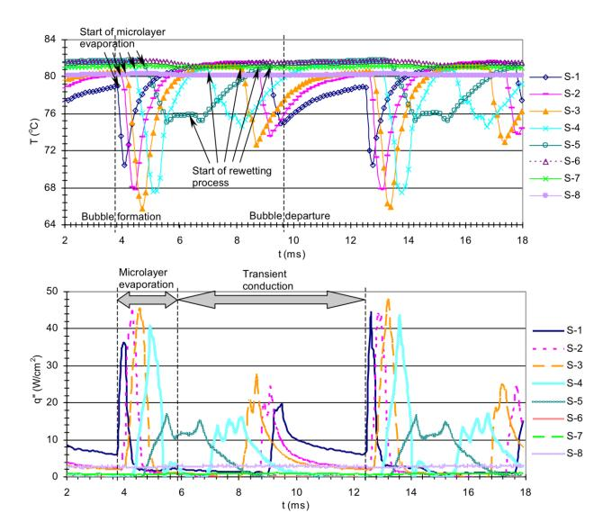
**Figure 7:** Surface temperature (upper panel) and heat flux (lower panel) variations during the bubbling event. Heat transfer during microlayer evaporation and transient conduction processes are marked. S-1 through S-8 indicate sensors 1-8 in Figure 5.
