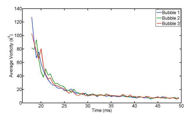
**Figure 2:** Post-processing of the PIV data in Figure 3 yields the values of the z-component of the vorticity vector in the wake of a steam bubble. The abscissa represents time after bubble nucleation (bubble departure occurs at t=16 ms). Maximum uncertainty for vorticity values is  $\sim 18\%$ . (from [51])
