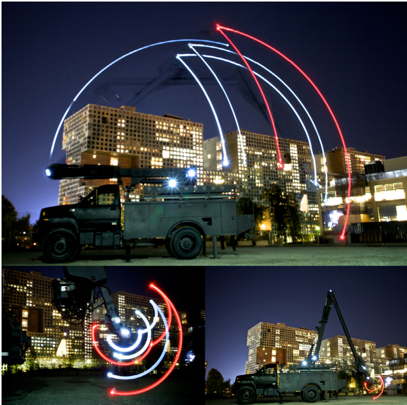
Figure 18-2. The range of motions for the DCP large (five-axis boom) and small (six-axis KUKA robot) arms are shown through long-exposure photography
