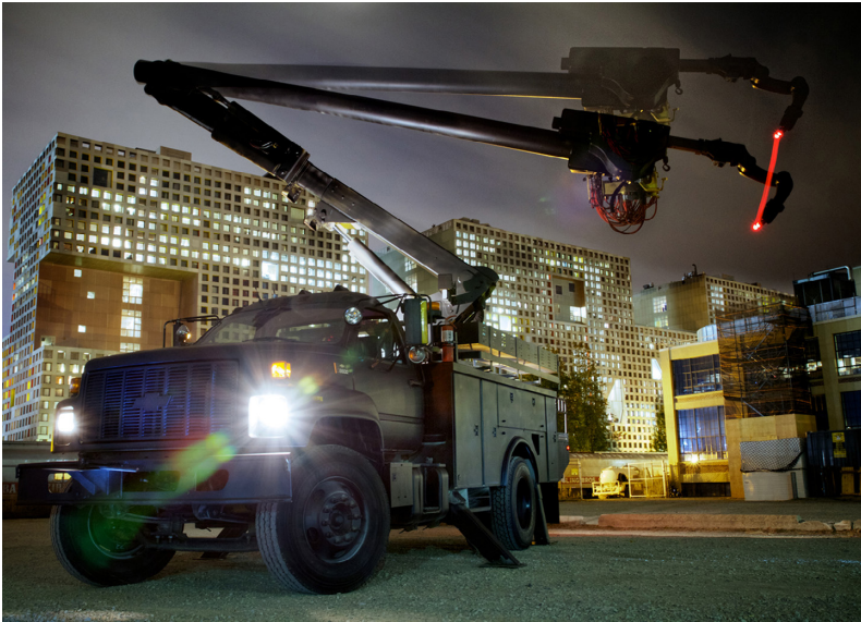
Figure 18-1. The Digital Construction Platform comprises a six-axis KUKA robotic arm mounted to a five-axis Altec hydraulic boom arm
