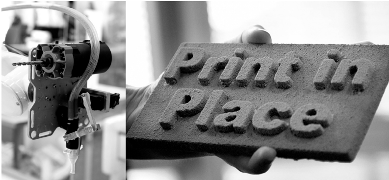
Figure 18-4. Combining additive and subtractive processes in a compound end effector (right) facilitates fast build times and high resolutions, as seen in the cast structure produced from a printed and milled mold
