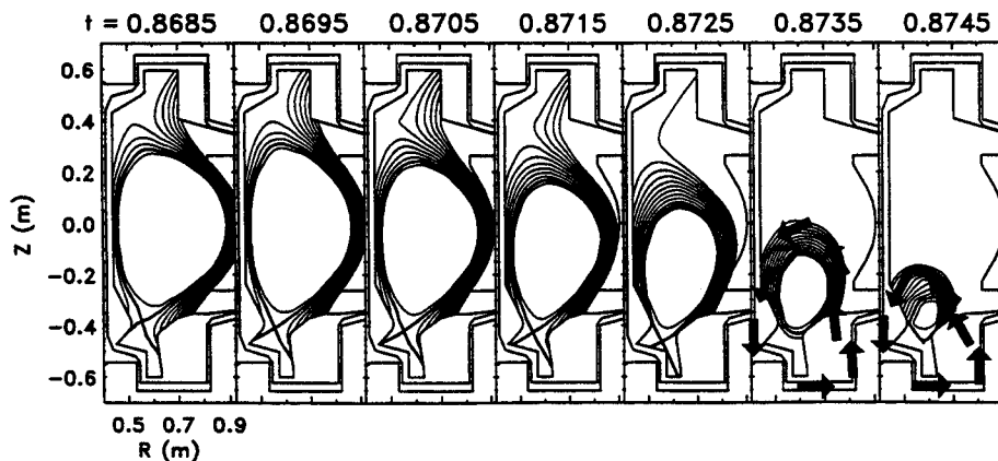
Figure 1 — Magnetic flux reconstructions at 1 ms intervals of a typical disruption. The arrows show the poloidal projection of halo current flow. The current path in the plasma scrape-off must actually be helical, in order to be force-free.
