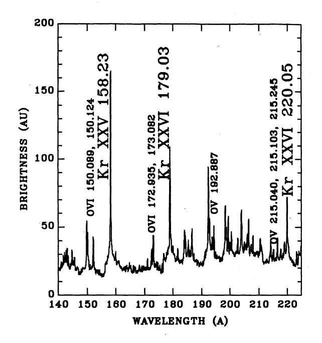
Figure 2. Composite Kr spectrum when enough Kr was puffed into the discharge so that  $Z_{eff}$ -1 due to Kr was ~ 0.1.
