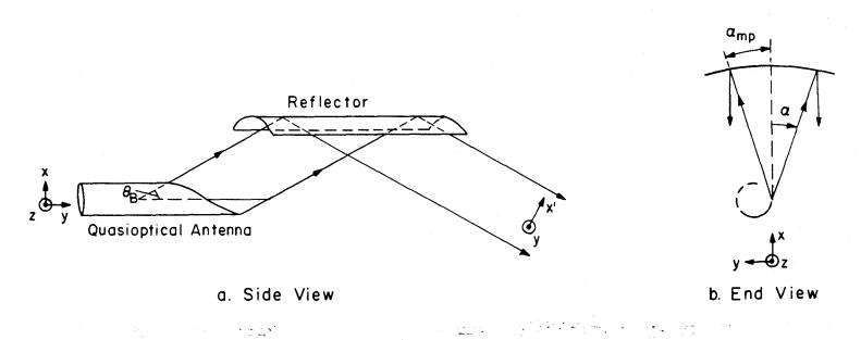
Fig. 4 Side and end view of a quasioptical antenna used in conjunction with the  $TE_{6,1,1}$  surface mode.
