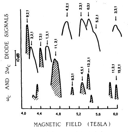
Fig. 5 Diode scan showing both fundamental (unshaded) and second harmonic (shaded) regions of operation.
