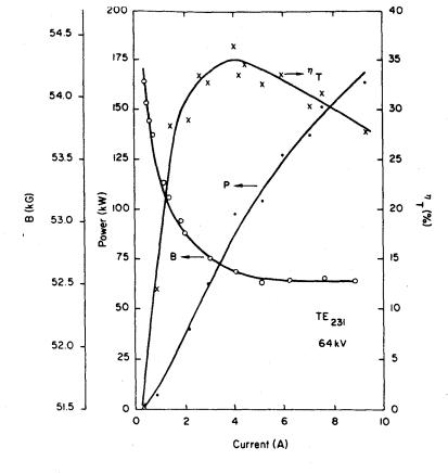
Fig. 1 Measured output power and total efficiency as a function of beam current for the  $TE_{2,3,1}$  mode. The magnetic field B has been optimized at each current.
