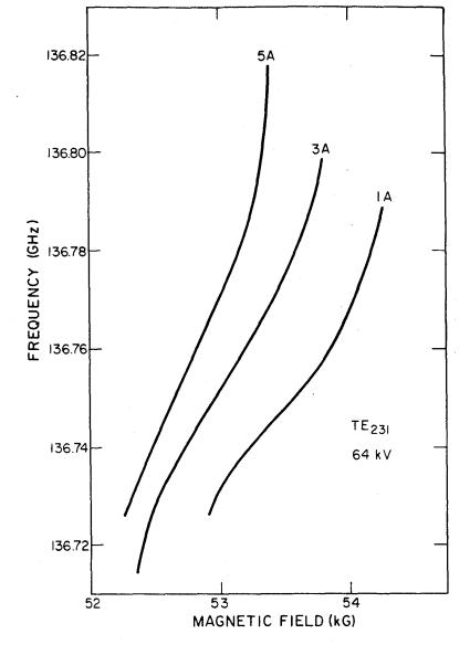
Fig. 3 Dependence of emission frequency on the beam current and magnetic field for the  $TE_{2,3,1}$  mode.
