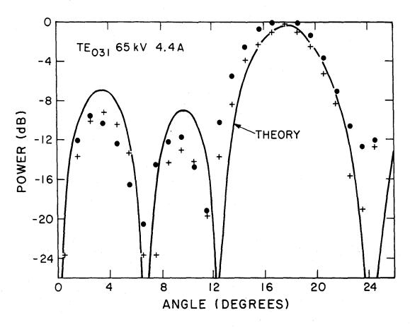
Fig. 2 Comparison of the theoretical and experimental far-field radiation pattern for the  $TE_{0,3,1}$  mode.
