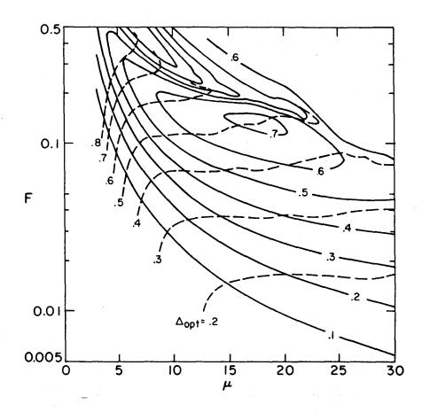
Fig. 6 Contour plot of the transverse efficiency (solid lines) and optimum detuning  $\Delta_{opt}$  (dashed lines) as a function of normalized field amplitude F and length  $\mu$ .
