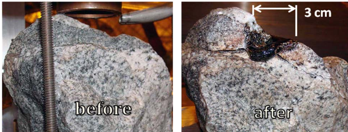
Figure 5. Before and after photos of third granite specimen with a non-flat surface showing the peaked ridged surface ablated away by the 28 GHz gyrotron beam.
