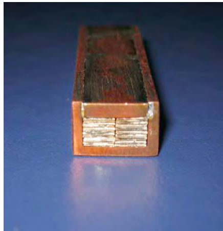
Figure 4. Untwisted cable developed at NIFS.
