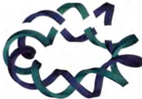
Fig. 12. Demountable (or segmented) HTS coils for helical devices.
