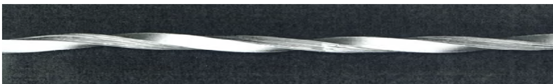
Fig. 3. Schematic illustrations of twisted stacked-HTS tape conductor.
