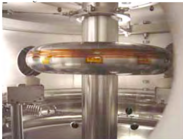
Fig. 17. Levitated coil in mini-RT experiment at the University of Tokyo.
