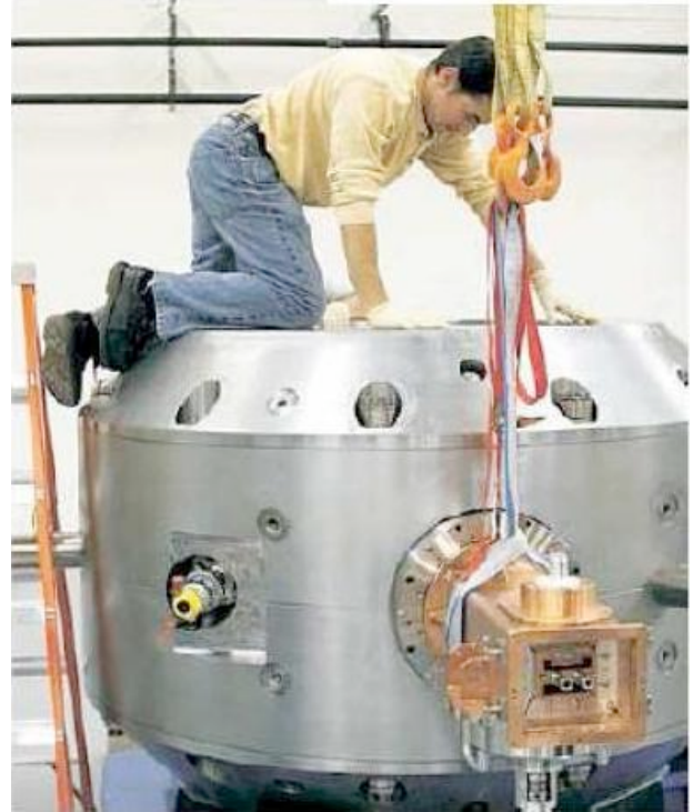
Fig. 28. A photo of the Still River Systems Monarch 250TM superconducting synchrocyclotron. The small size of this 250 MeV Proton machine is evident from the size of the man working on it.
