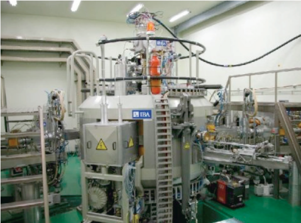
Fig. 20. The widely deployed IBA Cyclone 30 Isotope production cyclotron accelerates protons from 18-30 MeV, also simultaneously accelerating deuterons (9-15 MeV) and features dual isotope production targets.
