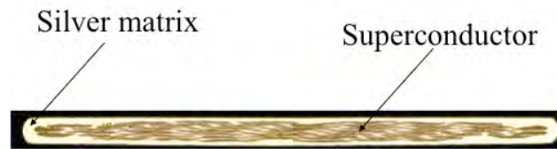
Figure 6. Cross section of “high current density” tape (BSSCO 2223) from American Superconductor Company.
