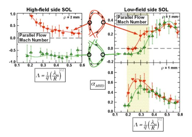
Fig. 4. Top left and right: Parallel Mach number on high ( $\rho$  =2 mm) and low-field side ( $\rho$  =1 mm) scrape-off layers as a function of  $\Lambda$ . Bottom right:  $\alpha_{MHD}$  versus  $\Lambda$ , evaluated at  $\rho$  =1 mm. Data points represent averages over all data shown in Figs. 2 and 3. USN discharges are seen to have lower  $\alpha_{MHD}$  values over range in  $\Lambda$  where flows in the low-field side SOL are also less co-current directed.
