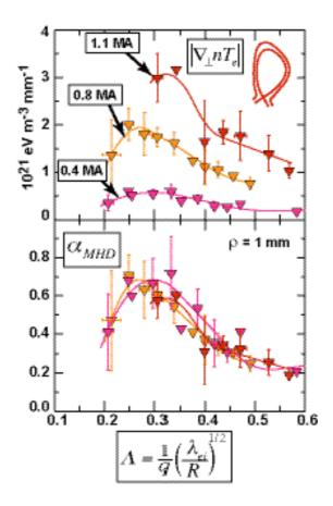
Fig. 2. Electron pressure gradients and  $\alpha_{MHD}$  versus  $\Lambda$  evaluated at  $\rho$  =1 mm for LSN discharges. Data points represent average values from a number of probe scans; error bars indicate typical ±1 standard deviation in data sample.
