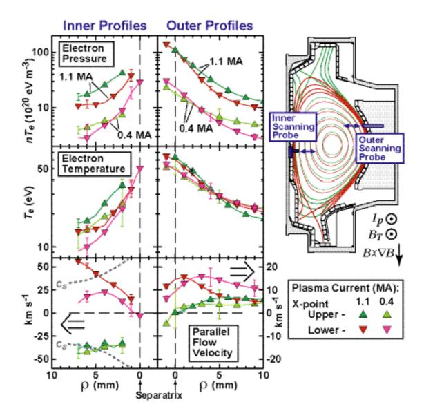
Fig. 1. Electron pressure, temperature and parallel plasma flow velocity profiles recorded from inner and outer scanning Langmuir-Mach probes for  $I_p = 1.1$  and 0.4 MA and 0.28 <  $\Lambda$  < 0.32 in matched LSN and USN discharges. Horizontal axis ( $\rho$ ) is distance outside the separatrix, mapped to the outer midplane. Positive velocities indicate a flow in the co-current direction; sound speed velocities ( $C_s$ ) are shown for reference.
