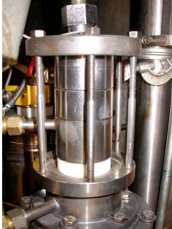
Figure 2. Photograph of the plasmatron used in these experiments, as well as those in reference [4-9].
