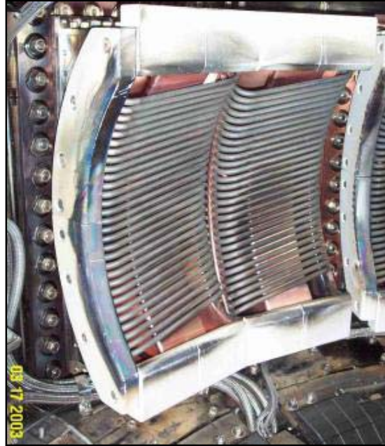
Figure 1: D antenna with BN (white) tiles installed.
