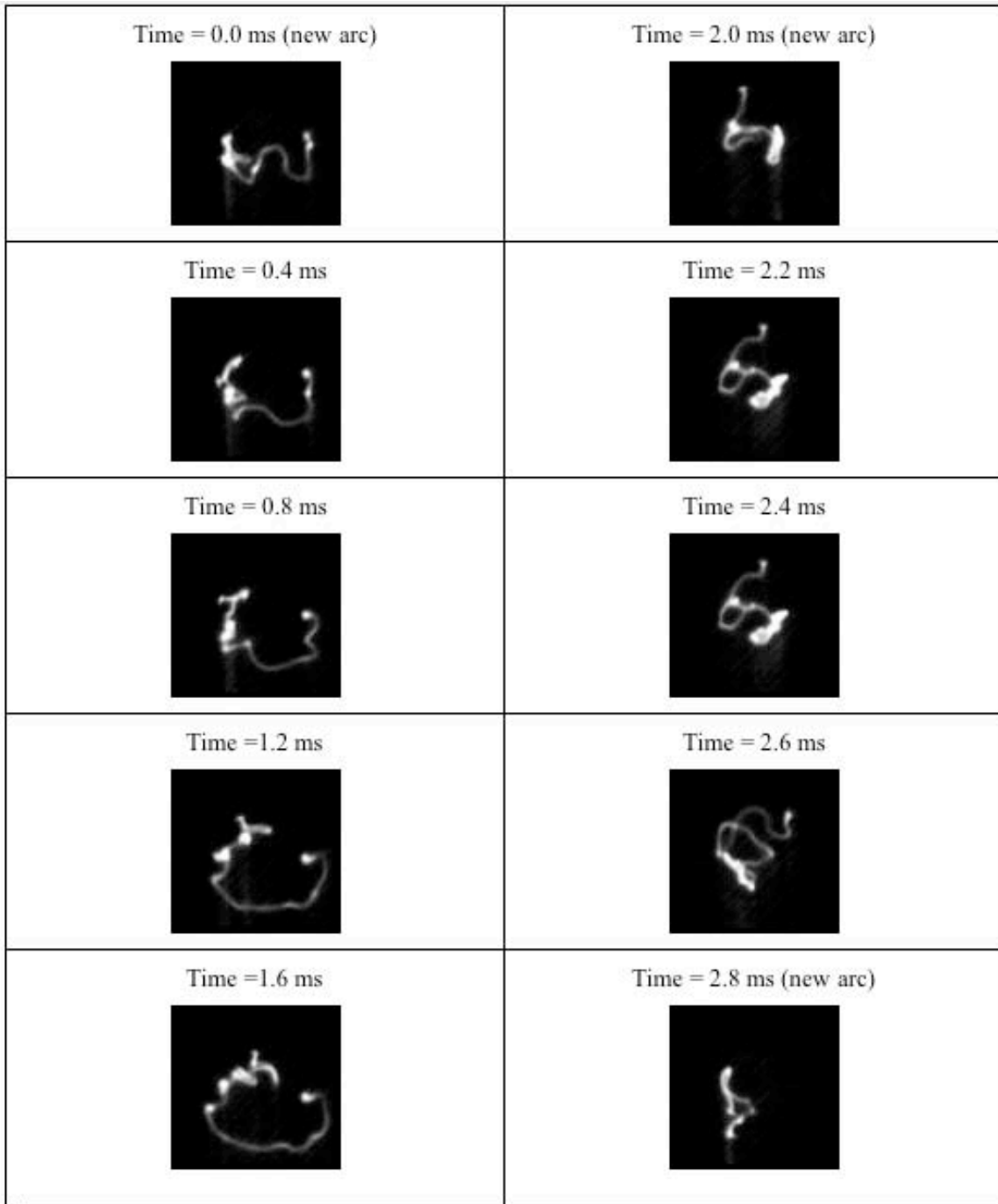
Figure 2. View of the Discharge Region along the y Direction from the Plasmatron Exit. The Sequence of Images along Time includes two Complete Discharges and a Third Arc Initiation
