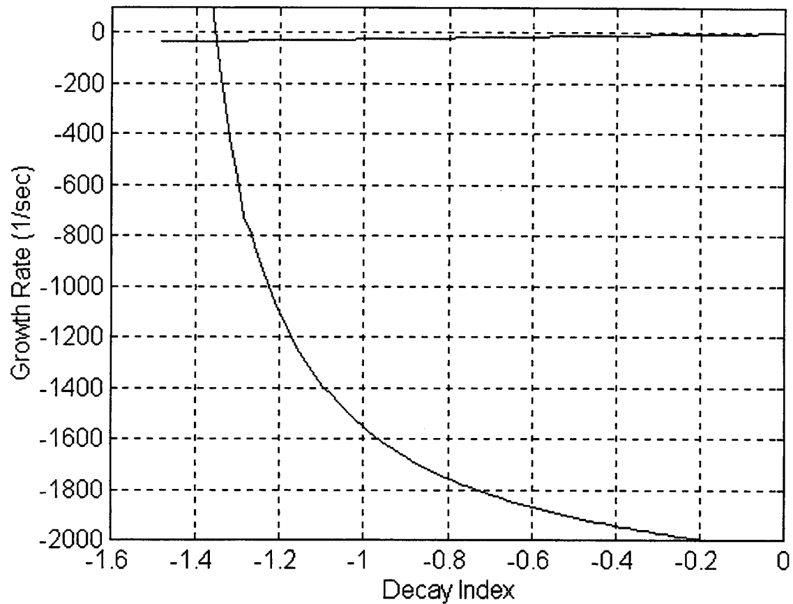
Figure 5.3 Plot of two growth modes as a function of decay index. The slower growth mode dominates the time response, but the second mode determines the point of instability. All robustness plots show the slowest growth mode, with a discontinuity on the graph when the second mode goes positive.
