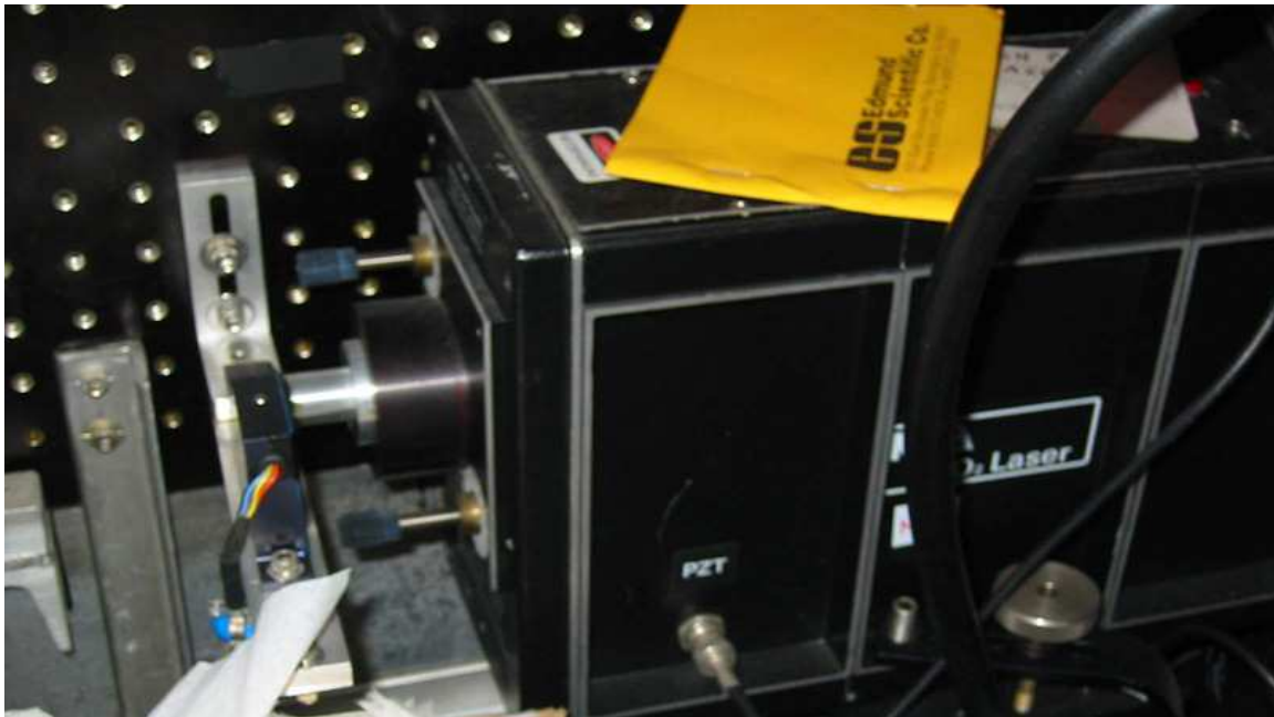
Figure 3-2: Photo of the DIII-D PCI laser and safety shutter.
