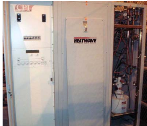
Figure 4. 10 kW, 28 GHz gyrotron system being installed at MIT PSFC.
