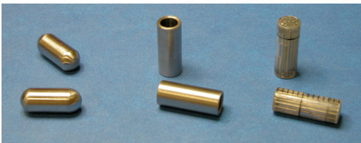
Fig. 4.1 Bullets from left: A. Rounded rod bullet (13.2 g) B. Hollow cylinder bullet (7.9 g) C. Wire assembly bullet (2.7 g)
