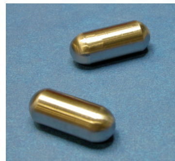
Rounded Rod Bullets (25 mm length, 10 mm Diameter)
