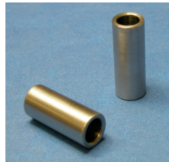
Hollow Cylinder Bullets (25 mm length, 10 mm OD, 7 mm ID)
