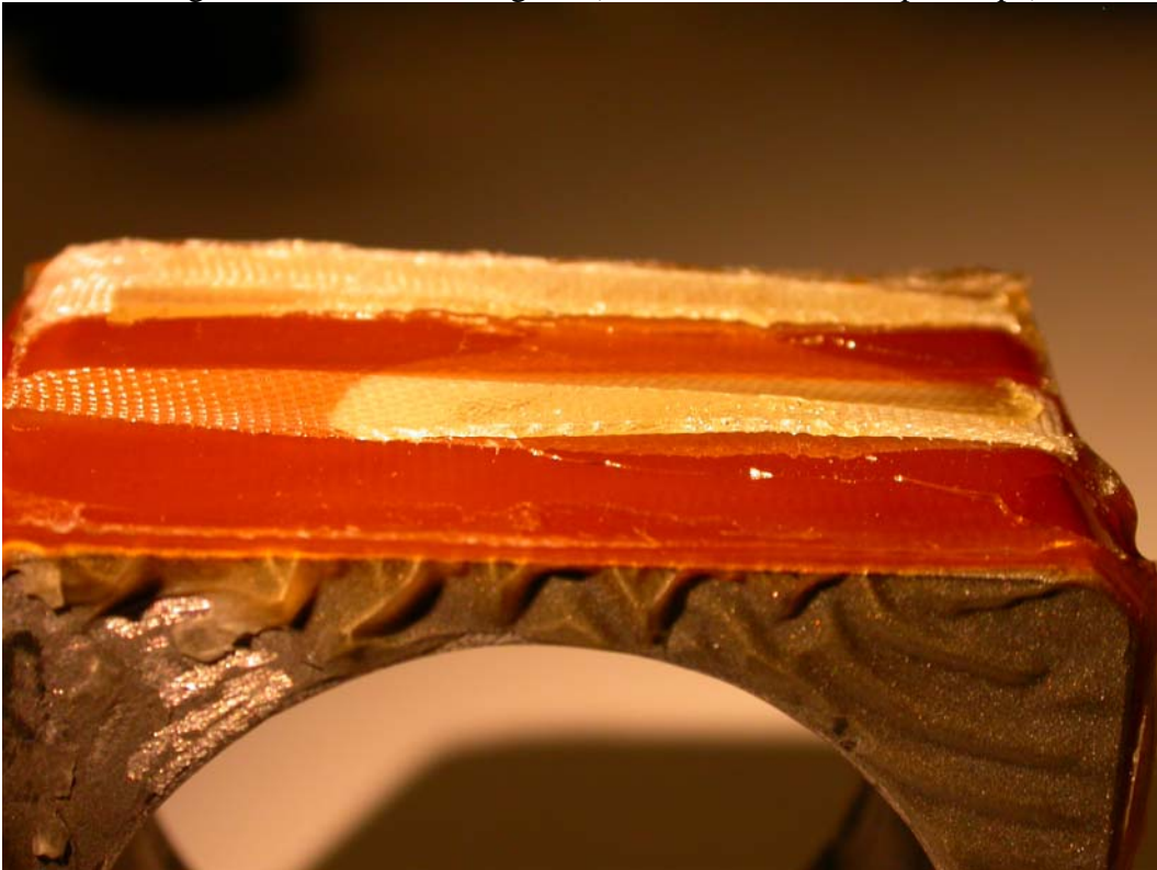
View showing delamination of fiberglass (with reflection on Kapton tape):
