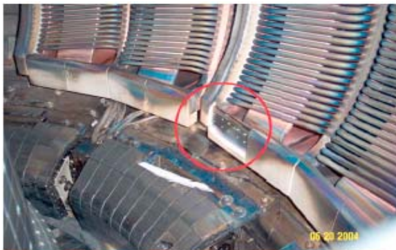
Figure 4 A fractured BN tile from the FY 2004 campaign.
