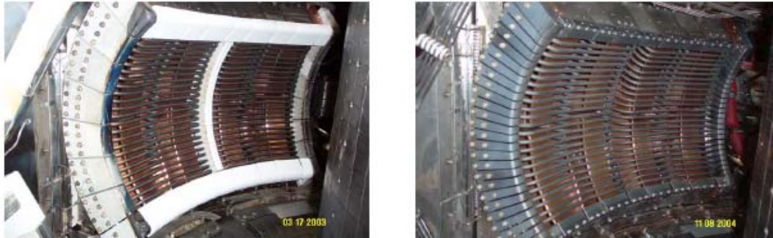
Figure 1 J antenna before and after the removal of BN tiles.
