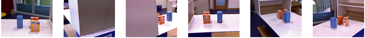
Figure 9: Examples of views from scenario 5. In all views except the final one, only one of the two orange baking-soda boxes was detected. This causes MHT to incorrectly infer that all measurements came from a single object (and prune other possibilities), whereas batch approaches such as clustering can revisit previous associations and correct them using new information, such as the final view where both boxes are finally detected.
