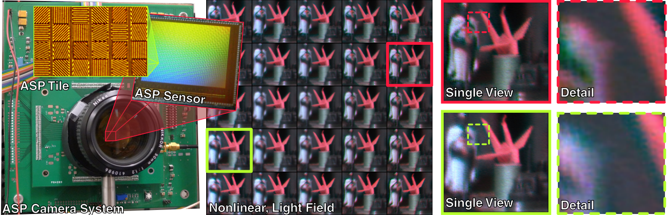
Figure 1: Prototype angle sensitive pixel camera (left). The data recorded by the camera prototype can be processed to recover a high-resolution 4D light field (center). As seen in the close-ups on the right, parallax is recovered from a single camera image.
