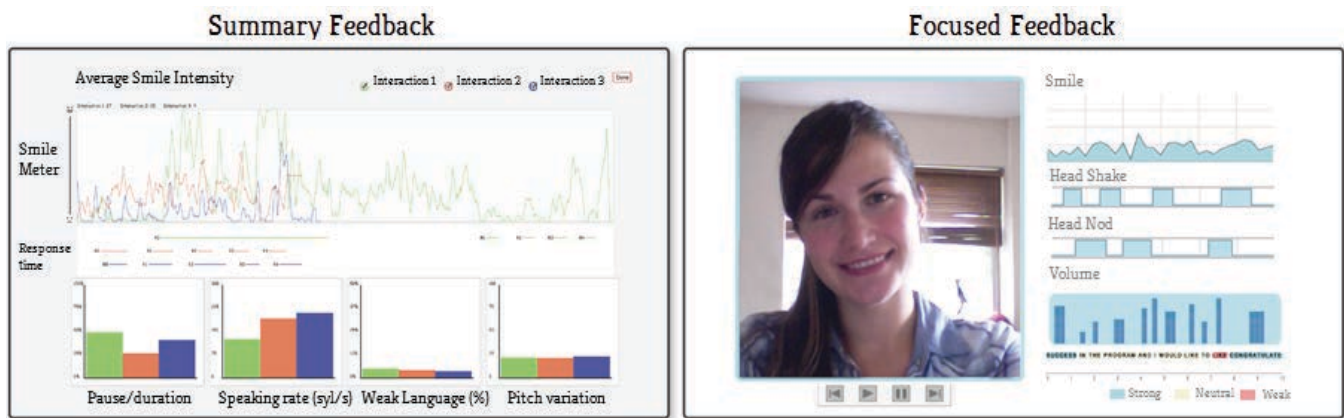
Figure 5. The two forms of feedback provided by MACH. The summary feedback (left) captures the overall interaction. Participants can practice multiple rounds of interviews and compare their performance across sessions. The focused feedback (right) enables participants to watch their own video. As they watch the video, they also can see how their nonverbal behaviors, such as smiles, head movements, and intonation change over time.
