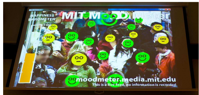
Figure 3. Example of the interface, as people interacted with one of the installations. Green blobs indicate faces detected as smiling, while yellow blobs indicate non-smiling faces.
