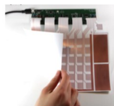
Figure 1. The PrintSense technique supports the development of multi-modal sensing arrays, printed as a single layer onto a flexible substrate and connected to a custom hardware module (left). It supports capacitive touch and proximity sensing along with resistive pressure sensing (centre) & bend sensing of the substrate (right).
