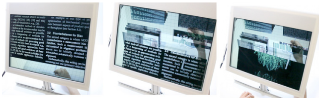
Figure 4. Users can spatially manage windows in 3D space, and leverage spatial memory to retrieve tasks.
