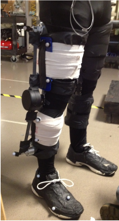
Fig. 4. Right leg instrumented for motion capture. Black tape covers all reflective surfaces.
