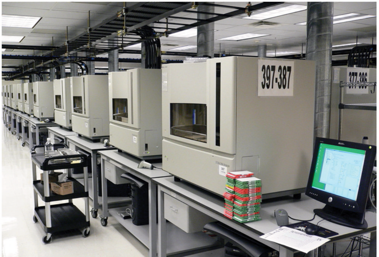
Figure 1. One of many rows of ABI 3730xl automated DNA Analyzers for shotgun sequencing of the human genome in months (30 billion bp/year) in 2005. (Courtesy: Steve Jurvetson)
