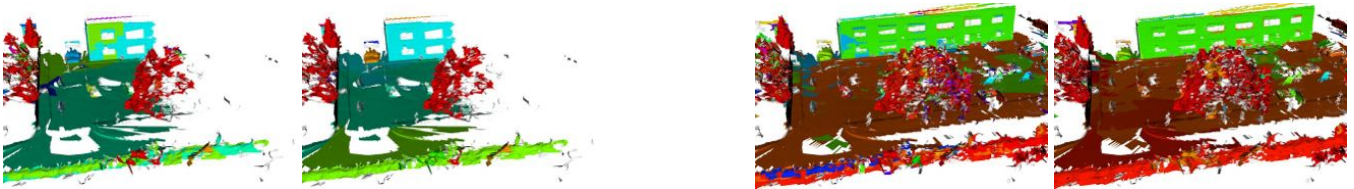
Figure 9: Effect of smoothing (best viewed in color) on two examples. Left image for each case shows the result using only online star clustering, the right image is the result after applying graph-based smoothing. As can be seen, class labels are clearer and distributed more precisely within each object.
