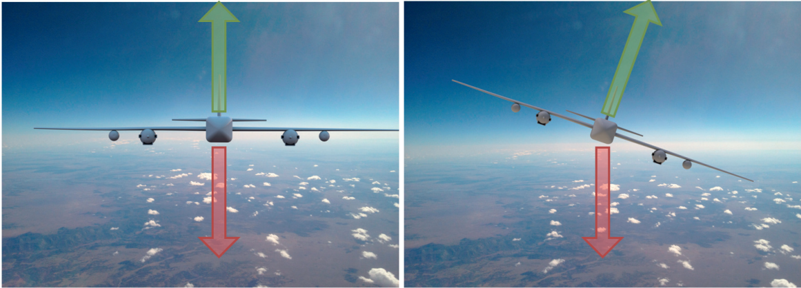
Figure 2. A vehicle (left to right): a) under steady level flight; and b) performing a standard rate turn. The weight of the aircraft (red arrow) is equal to the vertical component of the total aircraft lift (green arrow). The horizontal component of the total aircraft lift under b) creates a centripetal force, causing the aircraft to perform a turn.
