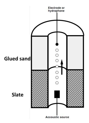
Figure 3: Diagram of the layered borehole model to measure the acoustic field and the seismoelectric field by fixing the acoustic source in the slate section and moving the electrode or acoustic hydrophone along the borehole and across the interface.
