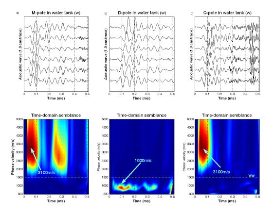
Figure 7: Acoustic waveforms and their semblance plots in the time domain when the multipole tool works in a water tank at (a) monopole, (b) dipole, and (c) quadrupole modes, respectively. The high-frequency signals received after 0.28 ms are the reflection from the boundary of the water tank. The source is excited by a single sine burst with 50 kHz in center frequency. The dotted line  $(V_w)$  indicates the water velocity.
