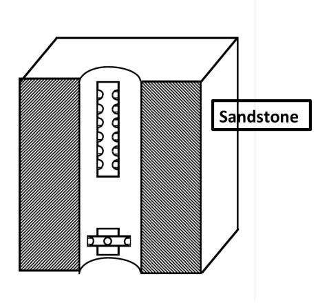
Figure 8: Schematic of the acoustic measurements in the sandstone borehole model with the tool without the connector between the source and receivers.
