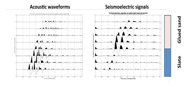
Figure 4: Acoustic waveforms (a) and seismoelectric signals (b) recorded in the borehole model (slate and glued-sand model) when the acoustic source is fixed in the slate section and the acoustic receiver or electrode moves from the slate section to glued-sand section. The fifth trace is located at the interface.
