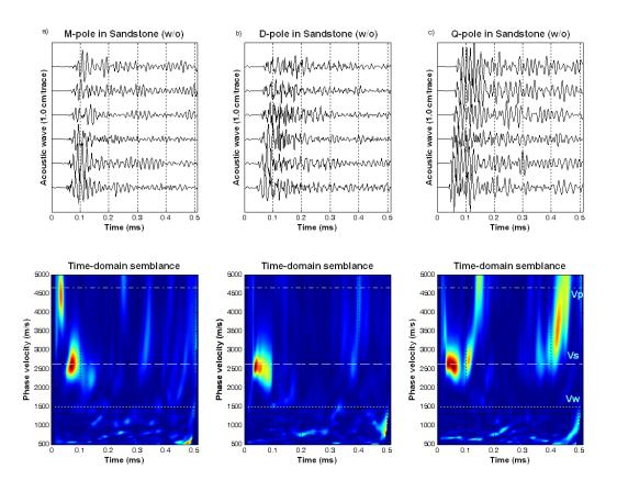
Figure 9: Acoustic waveforms and their semblance plots in the time domain when the multipole tool works in the sandstone borehole model at (a) monopole, (b) dipole, and (c) quadrupole modes without the connector, respectively. The dotted-dashed line  $V_p$  and the dashed line  $V_s$  indicate the P- and S-wave velocities in sandstone, respectively. The dotted line  $V_w$  indicates the water velocity.
