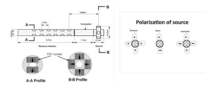
Figure 5: Schematic of a scaled multipole acoustic logging tool with a source and six receiver pairs. The single transducer is a PZT cylinder crystal that is 0.64 cm in diameter and 0.37 cm long. The radiation patterns are shown on the right side when the source works as monopole, dipole, and quadrupole, respectively.
