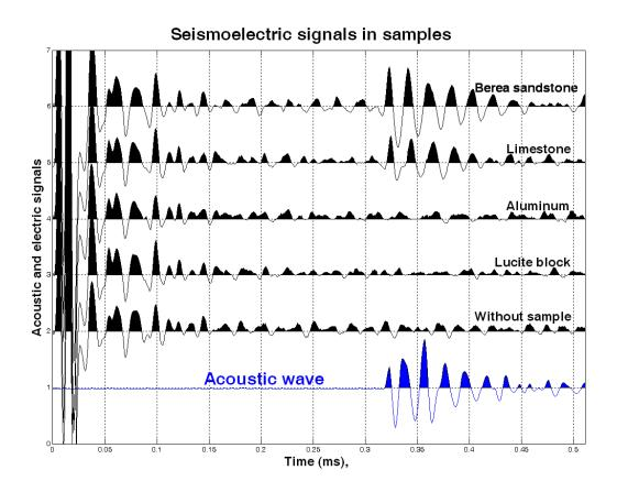
Figure 2: Acoustic waveform (trace 1 with the blue line) and electric signals measured with the different samples. Trace 2 is the electric signal recorded with the electrode when there is no sample. Other traces show electric signals recorded when samples are Lucite (trace 3), aluminum (trace 4), limestone (trace 5), and Berea Sandstone (trace 6), respectively.
