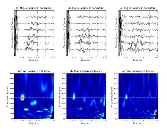
Figure 14: Seismoelectric signals and their semblance plots in the time domain when the multipole seismoelectric tool works in the sandstone borehole model as (a) monopole, (b) dipole, and (c) quadrupole modes, with the connector between the source and receiver sections, respectively. No electric signals with the apparent velocity of the tool wave are recorded. The horizontal lines of  $V_p$ ,  $V_s$ , and  $V_w$  indicate the P-wave, S-wave and water velocities, respectively.
