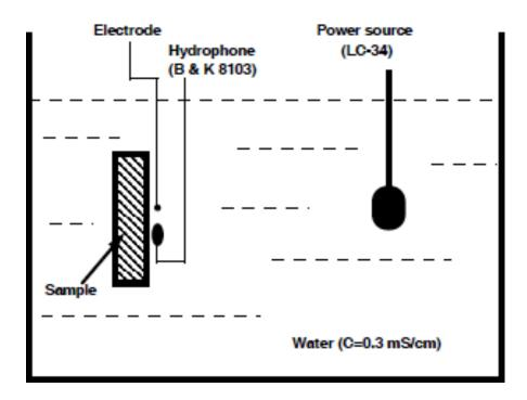
Figure 1: Schematic of seismoelectric measurements in a water tank. A single sine burst with 150V and 70 kHz excites the source hydrophone (Celesco LC-34). Measurement electrode records the electric potential close to the sample surface. A receiver hydrophone (B & K 8103) is placed near the sample to measure the acoustic wave arriving at the sample.
