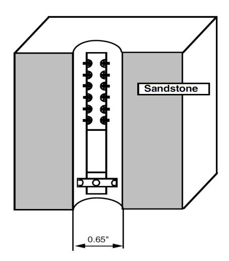
Figure 13: Schematic of the seismoelectric measurements in the sandstone borehole model when the tool is tightly connected with the connector between the source and receivers.
