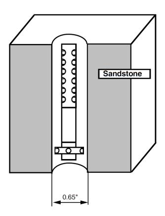
Figure 10: Schematic of the acoustic measurements in the sandstone borehole model when the tool it tightly connected with the connector between the source and receivers.
