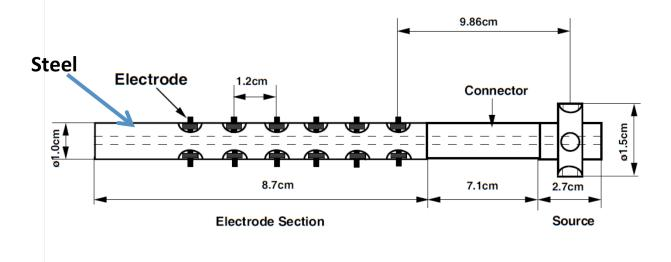
Figure 12: Schematic of a scaled multipole seismoelectric logging tool with a source and six electrode pairs. The receiver crystals in Figure 5 are replaced with the electrodes. The source and the tool sizes are the same as the tool shown in Figure 5.
