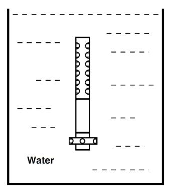
Figure 6: Schematic of the acoustic measurements in a water tank when the source and receiver section are tightly connected to simulate acoustic LWD tool.
