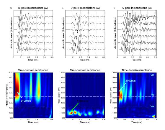
Figure 11: Acoustic waveforms and their semblance plots in the time domain when the multipole tool works in the sandstone borehole model (a) monopole, (b) dipole, and (c) quadrupole modes, with the connector between the source and receiver sections, respectively. The strong tool waves are recorded in the three modes. The horizontal lines of  $V_p$ ,  $V_s$ , and  $V_w$  indicate the P-wave, S-wave and water velocities, respectively.
