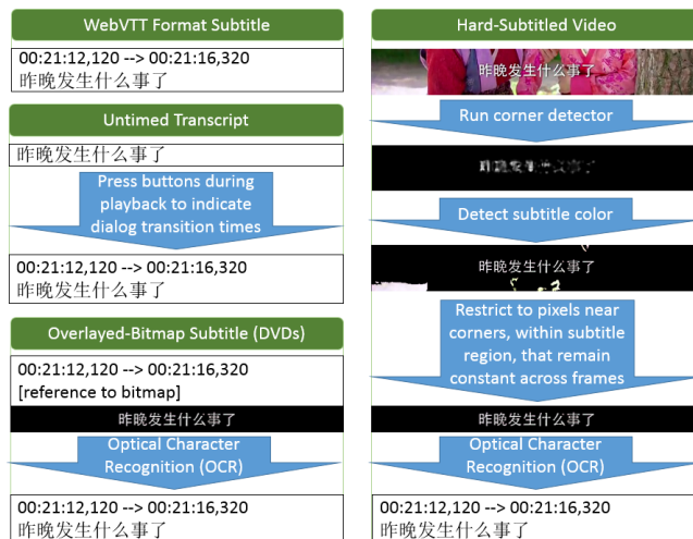
Figure 4. An overview of the sources that the Smart Subtitles system can extract subtitles from, and what the process of subtitle extraction consists of for each source.
