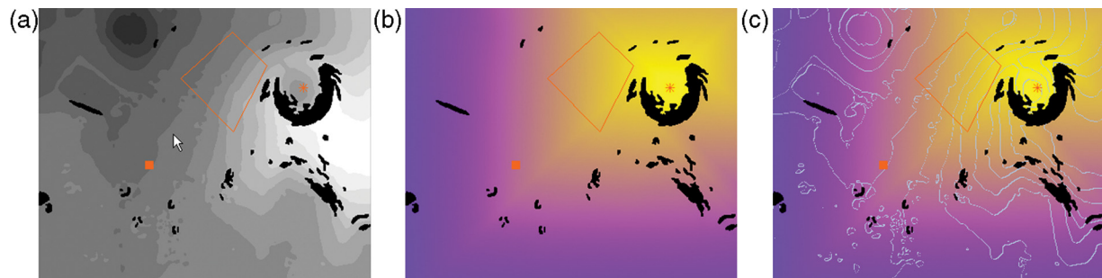
Fig. 2 Possible map visualizations, including start & goal locations and designated way-area; a) elevation contours visualization, b) levels of equal cost visualization, and c) both visualizations.
