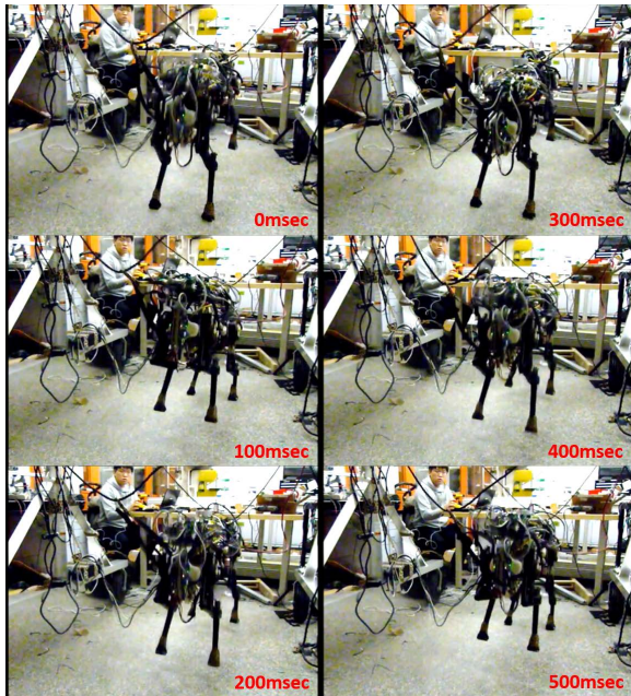
Fig. 10. Snapshots of bounding with duty ratio of 0.36 ( T_{\text{stance}} = 80 msec and T_{\text{swing}} = 220 msec) at intervals of 100 msec. The snapshots progress temporally from top to bottom, and then left to right.
