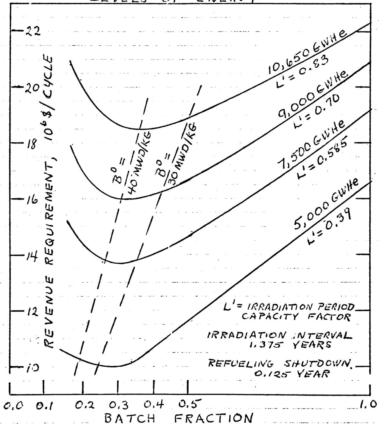
FIG. 1.7 OPTIMAL BATCH FRACTION VS
