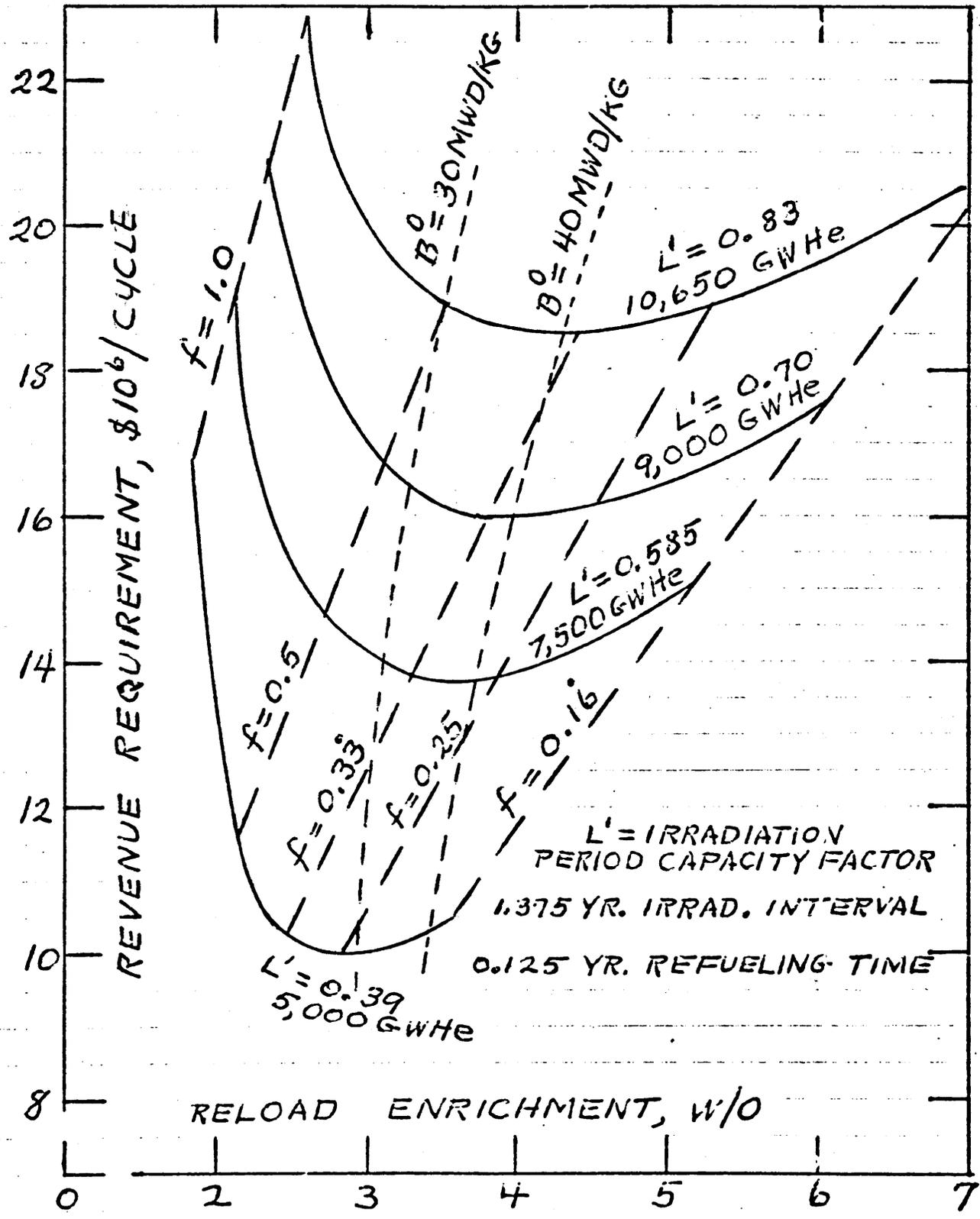
The calculation of incremental cost of energy for the case of variable reload enrichment and batch fraction deserves special attention. According to Equations (1.4) and (1.4a)  $\lambda$  is given as
