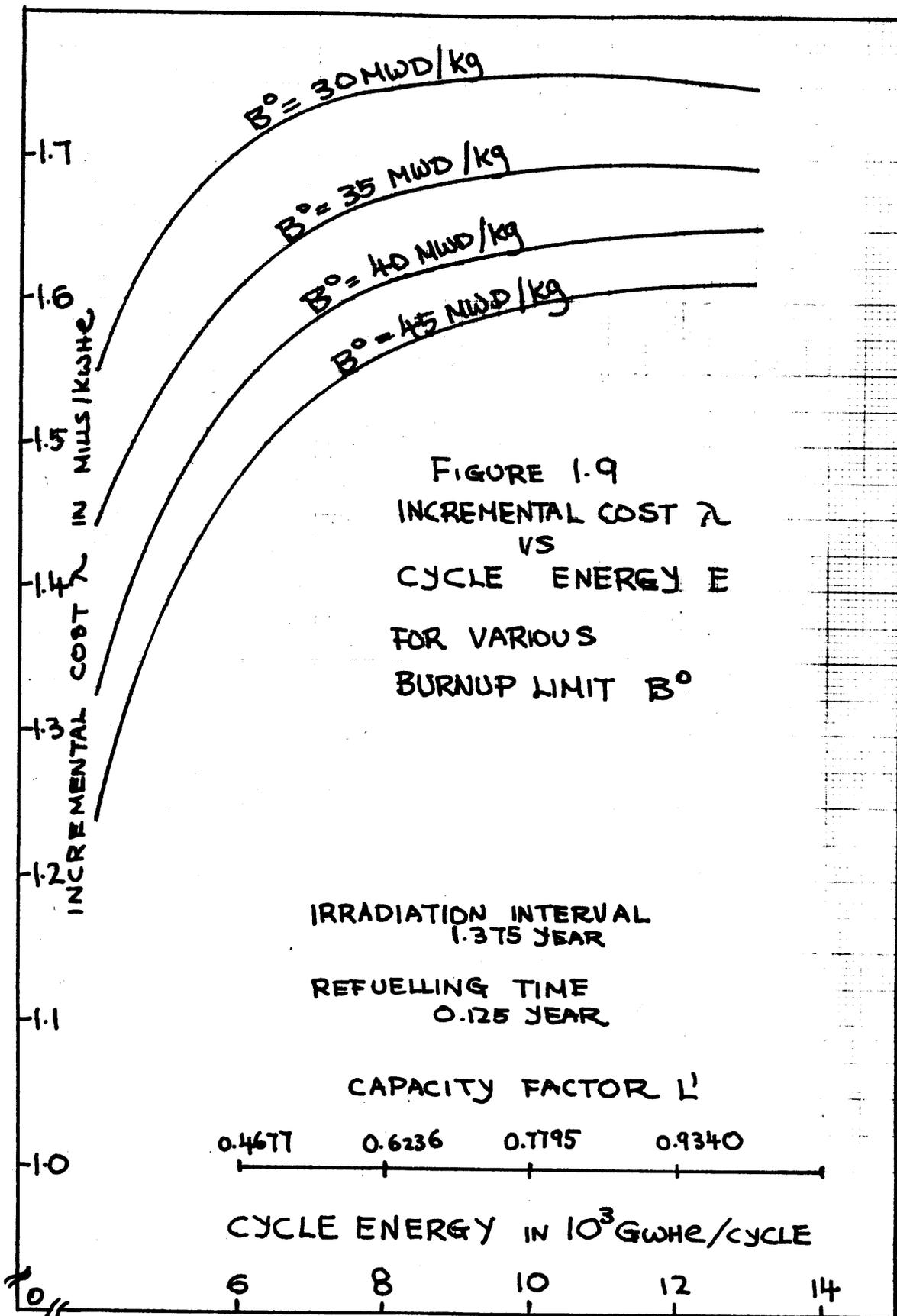
cost of energy versus cycle energy for different values of burnup limits. Initially, incremental cost increases rapidly with respect to cycle energy but gradually levels off. As the burnup limit decreases, incremental cost increases.
