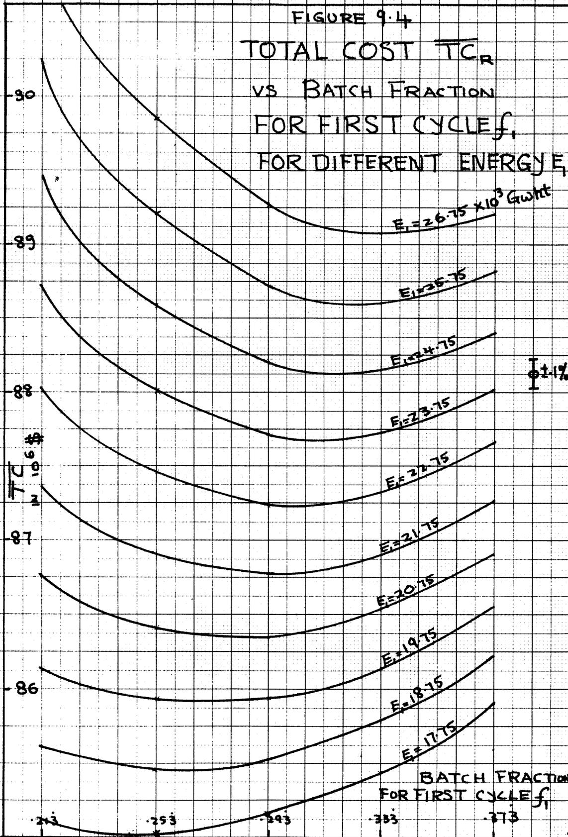
trend of higher optimal batch fraction at higher cycle energy is illustrated more clearly. Refer to Figure 6.5 for comparisons between steady-state and non-steady state results.
