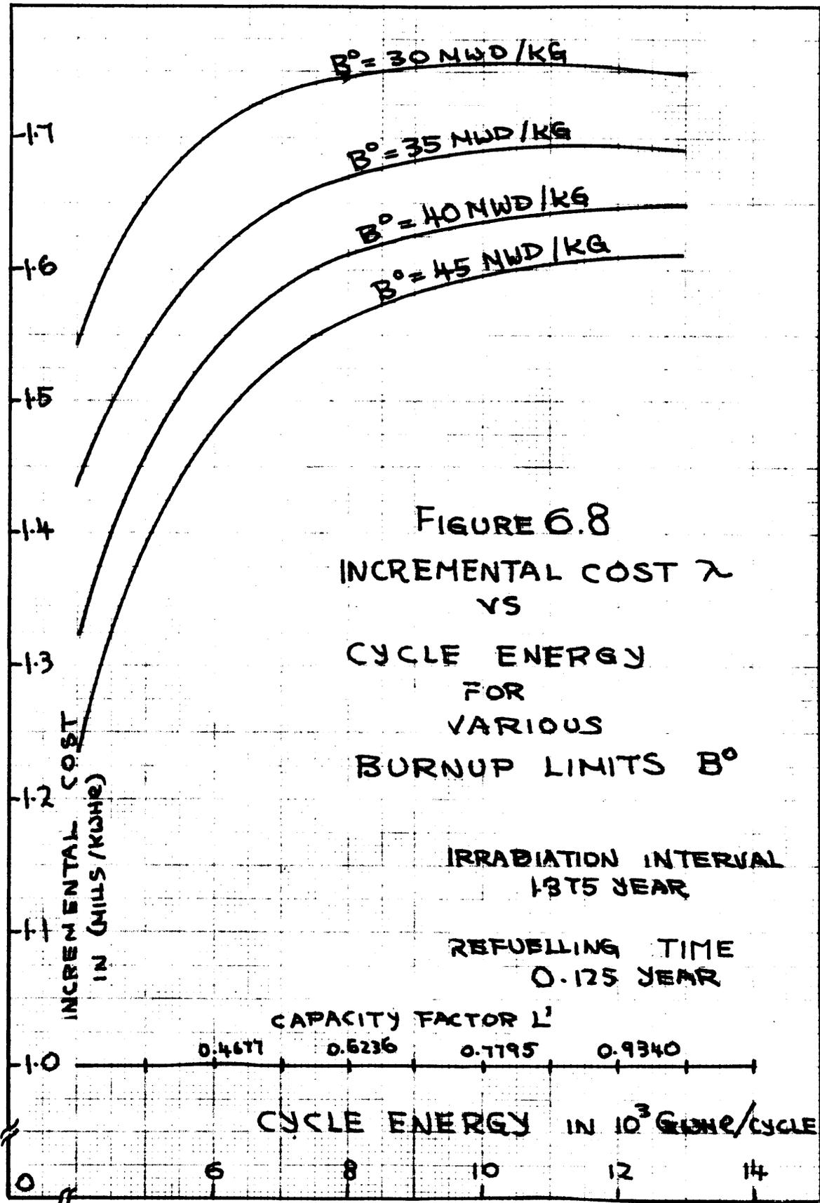
decreasing allowable burnup levels. For the same burnup, incremental cost first increases, then levels off and finally decreases for increasing cycle energy.
