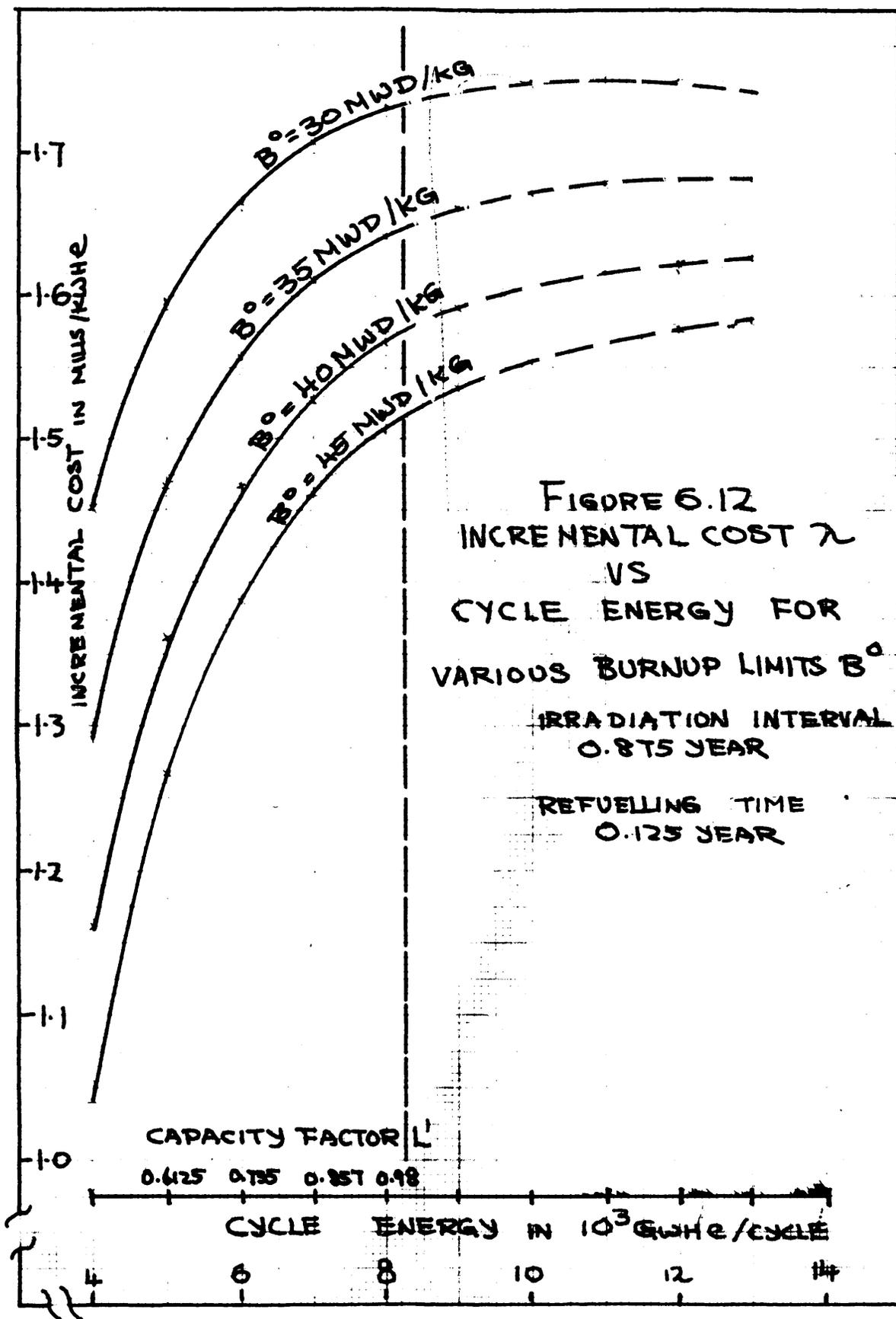
costs resulting from a smaller batch fraction outweighs the additional enrichment cost, carrying charges and income taxes. Finally, the incremental cost of energy increases with cycle energy, but levels off at  $E^S \approx 10,000$  GWHe/cycle. The incremental cost of energy also increases with decreasing allowable burnup levels.
