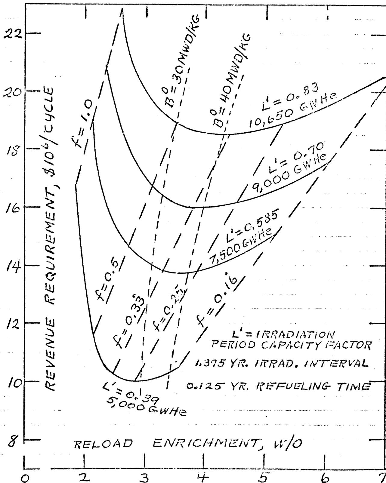
Decreasing batch fraction by  $\partial f$  would result in a saving of  $\frac{\partial \overline{TC}(E^S, f^*)}{\partial f} \cdot \partial f$  dollars
