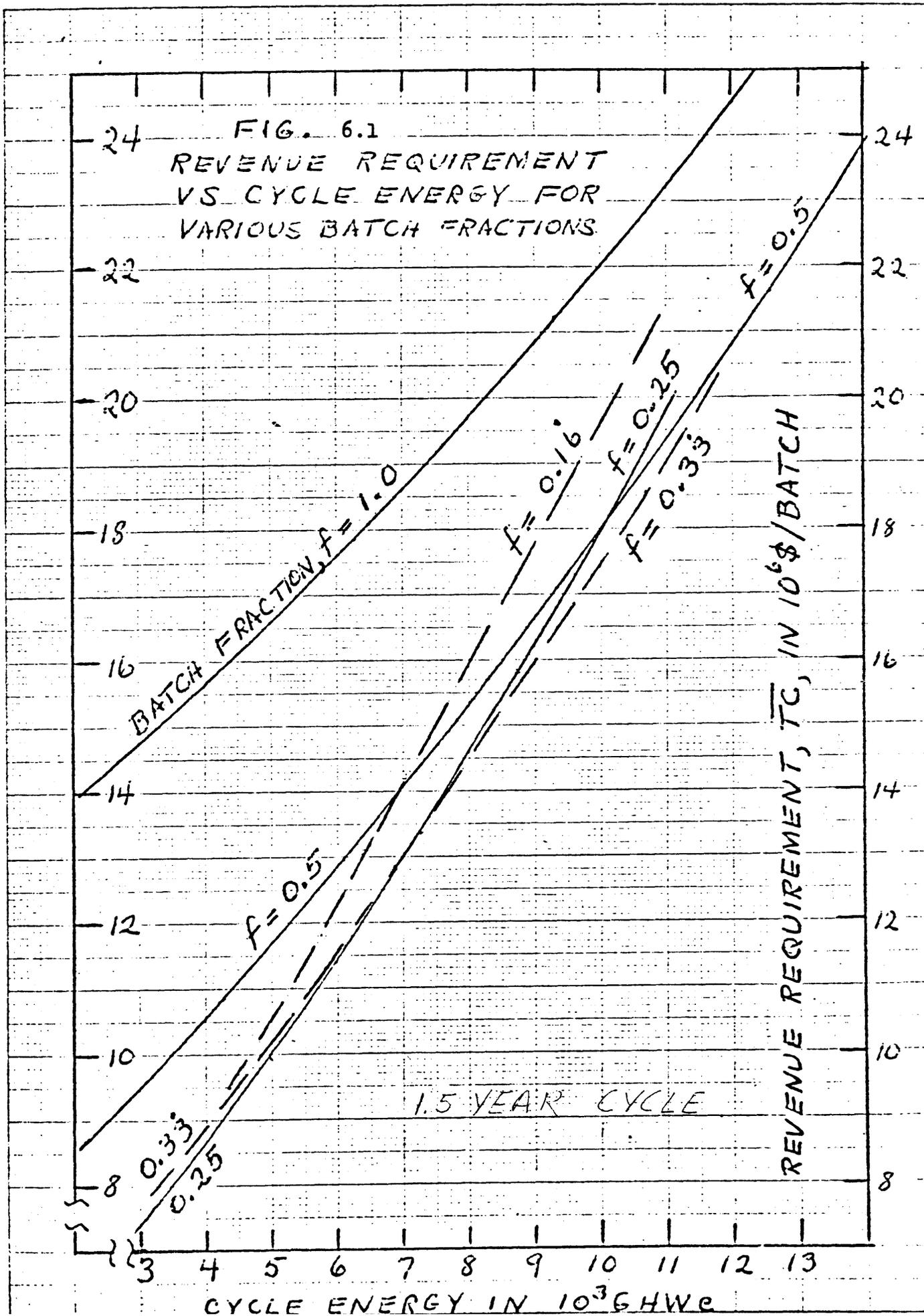
Figure 6.2 shows the variation of revenue requirement with respect to batch fraction for various cycle energies. The curves are rather flat near the minimum. Hence, in the vicinity of the minimum, economics plays a less important role than engineering and physical considerations.
