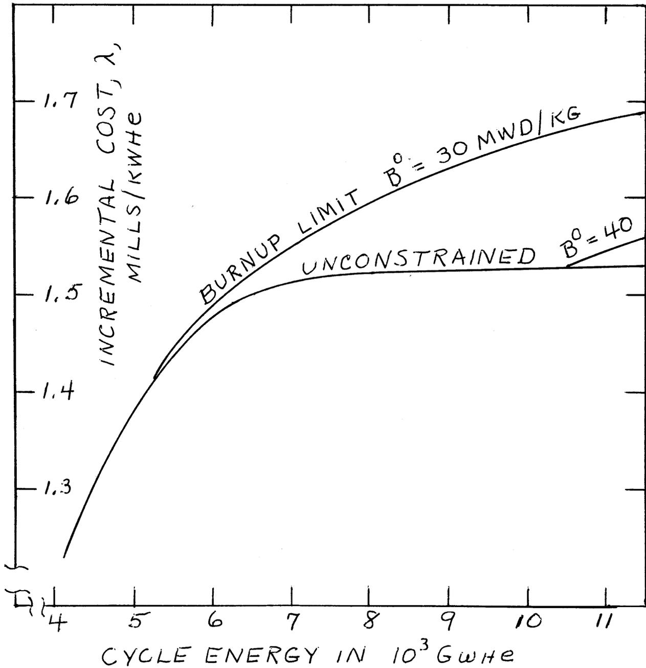
decreasing allowable burnup levels. When the burnup constraint is not controlling, incremental cost first increases, then levels off with increasing cycle energy.
