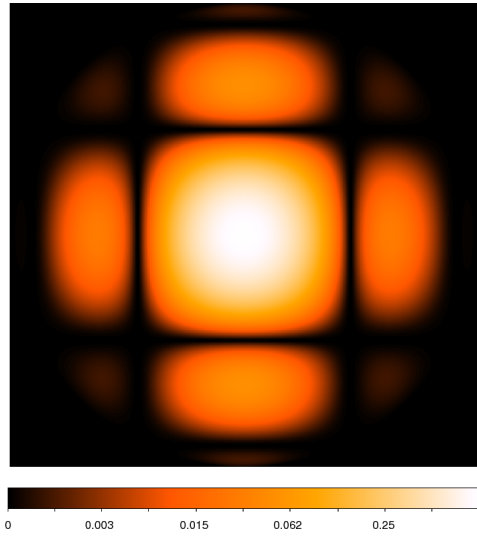
Figure 7: Simulated beam response for a single MWA tile, as described in the text.
