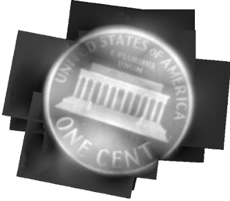
Fig. 6. Tactile map of the surface of a penny created by registering several partial tactile images into a single height map.
