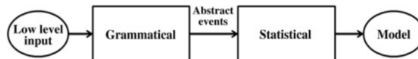
Fig. 3 A combined grammatical and statistical approach infers future behavior from a stream of current behavior.
