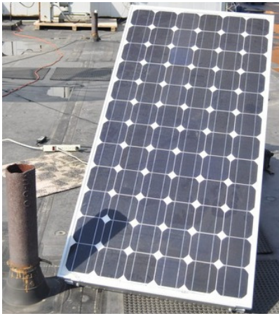
Fig. 11. Photograph illustrating the shading (owing to a protruding pipe) that moves across the panel for the dynamic performance experiment.
