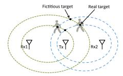
**Figure 3—Challenge in Localizing Multiple People.** The figure shows what happens when we have the same setup as Fig. 1(d) but add a second person to the scene. We get two TOF measurements at each Rx, which results in four ellipses having four intersection points within the beam of the antennas. Only two of these intersections are real targets, and the other two are fictitious targets.
