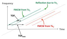
**Figure 6—Multi-shift FMCW**. WiZ transmits FMCW signals from different transmit antennas after inserting virtual delays between them. This delay must be larger than the highest time-of-flight (*TOF*<sub>limit</sub>) due to objects in the environment.
