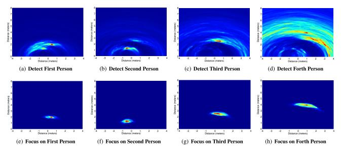
**Figure 8—Successive Silhouette Cancellation.** (a) shows the 2D heatmap obtained by combining all the TOFs in the presence of four users. (b)-(d) show the heatmaps obtained after cancelling out the first, second, and third user respectively. (e)-(h) show the result of the SSC focusing step on each of the person, and how it enables us to accurately localize each person while eliminating interference from all other users.
