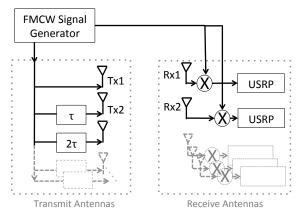
**Figure 7—Multi-shift FMCW Architecture.** The FMCW generated FMCW signal is fed to multiple transmit antennas via different delay lines. At the receive side, the TOF measurements from the different antennas are combined to obtain the 2D heatmaps.
