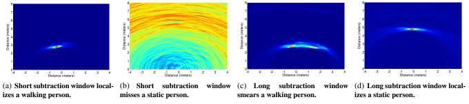
**Figure 11—Need For Multiple Subtraction Windows.** The 2D heatmaps show that a short subtraction window allows WiZ accurately localize a pacing person in (a) but not a static person in (b). A long subtraction window would smear the walking person's location in (c) but allows WiZ to localize a breathing person in (d).
