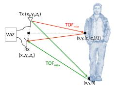
**Figure 9—Finding**  $TOF_{min}$  **and**  $TOF_{max}$ .  $TOF_{min}$  is determined by the round-trip distance from the Tx-Rx pair to the closest point on the person's body – i.e., the projection of the midpoint of [Tx,Rx] on the person's body. Since the antennas are elevated,  $TOF_{max}$  is typically due to the round-trip distance to the person's feet.
