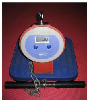
Gambar 5. Leg Dynamometer
