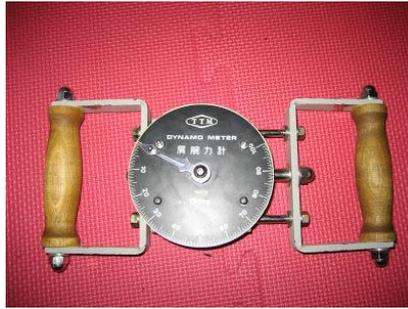
Gambar 6. Hand Dynamometer
