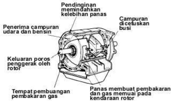
Gambar 15. Mesin rotary wankel
