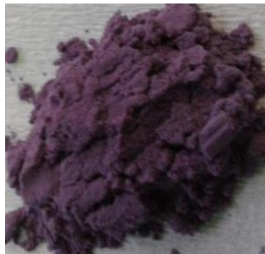
Gambar 5.1 Produk senyawa kompleks Cr-glu ( [\text{Cr}(\mu\text{-OH})(\text{glu})(\text{OH})_2]_2 \cdot 6\text{H}_2\text{O} )
