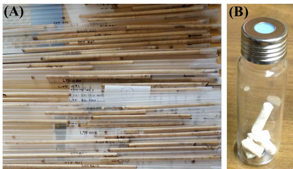
Figure 6: Core samples after removal from the tree-corer extractor and storage in (A) plastic straws for dendrochronological and dendrochemical analyses and (B) A glass screw-top 20 mL vial for phytoscreening, and transported to the North West River Research Station of the Labrador Institute. (Figure prepared by Sean Murphy).
