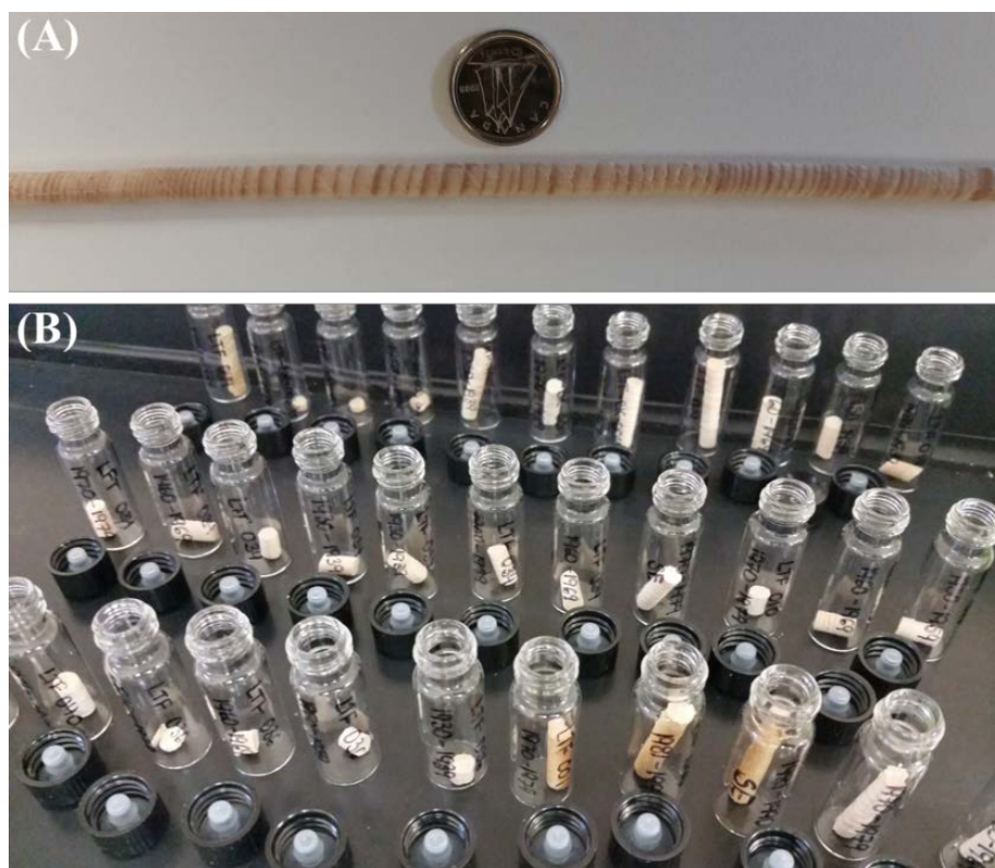
Figure 7: Tree-core sample for dendrochemical analysis. (A) A tree core prepared and ready for age dating. (B) Selected 9-year core segments in 4 mL glass vials to send for the analysis of major and trace elements by HR-ICP-MS. Note the variations in widths of annual tree rings and in the size of the core segments. (Figure prepared by Sean Murphy).
