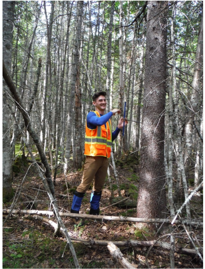
Figure A6: Sean Murphy screwing the tree corer in a black spruce tree to collect a core sample.
