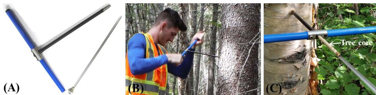
Figure 5: Tree-core sampling process. (A) The tree-corer used in this study, also known as an increment borer (the T-shaped metal instrument), and the tree-core extractor device. (B) The tree corer is drilled through the center of the trunk of the tree by pressing the tip of the corer firmly against the bark of tree trunk and turning the handles clockwise. (C) The extractor device is inserted into the corer from the handle end to carry and pull out the tree-core sample, a small cylinder of wood from the tree; the corer is withdrawn from the tree by turning the handle in counter clockwise direction. (Figure prepared by Sean Murphy).
