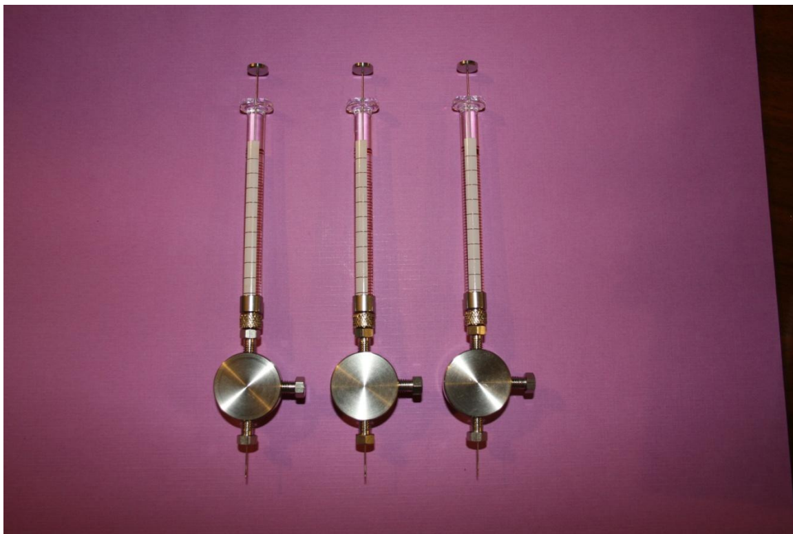
Figure B-3 Configuration for continuous flow single-drop extraction using three sets simultaneously.
