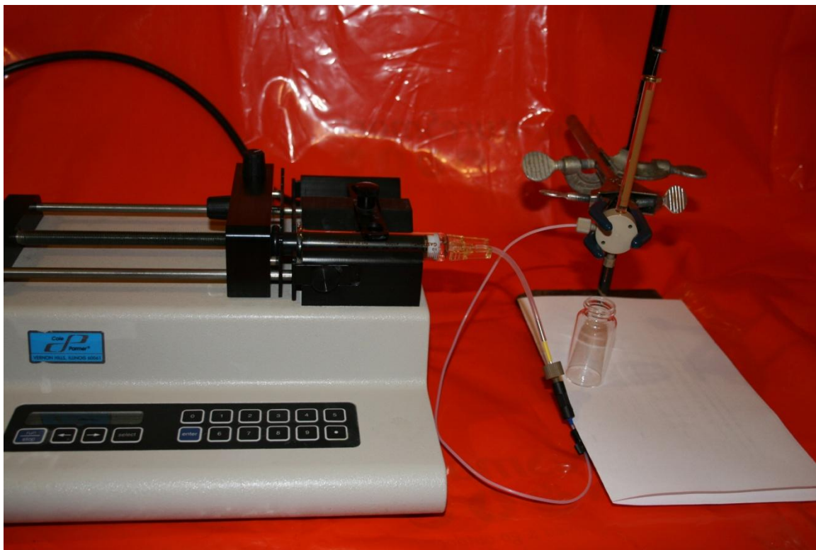
Figure B-3 Configuration for continuous flow single-drop extraction using syringe pump.
