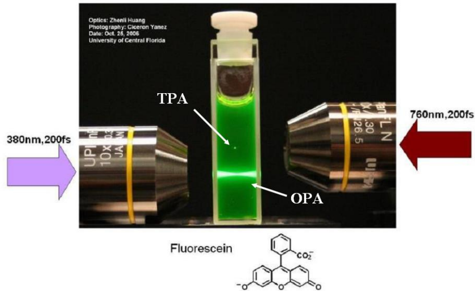
Figure 1-2 Observation of fluorescence excitation through the path of a laser beam
