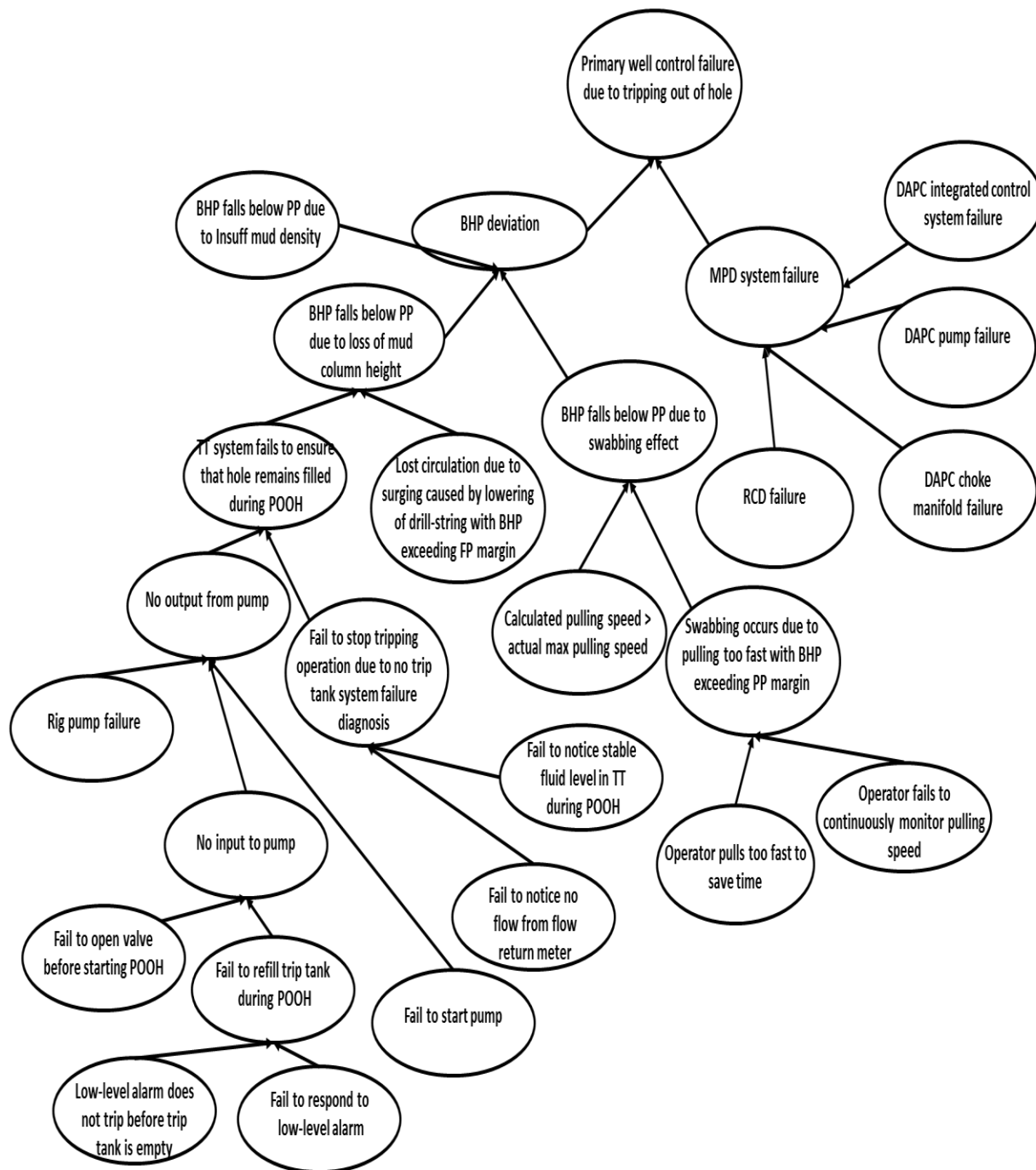
Figure 9.5 – Bayesian Network equivalent of tripping-out operation in CBHP technique of MPD (Abimbola, et al., 2015b)
