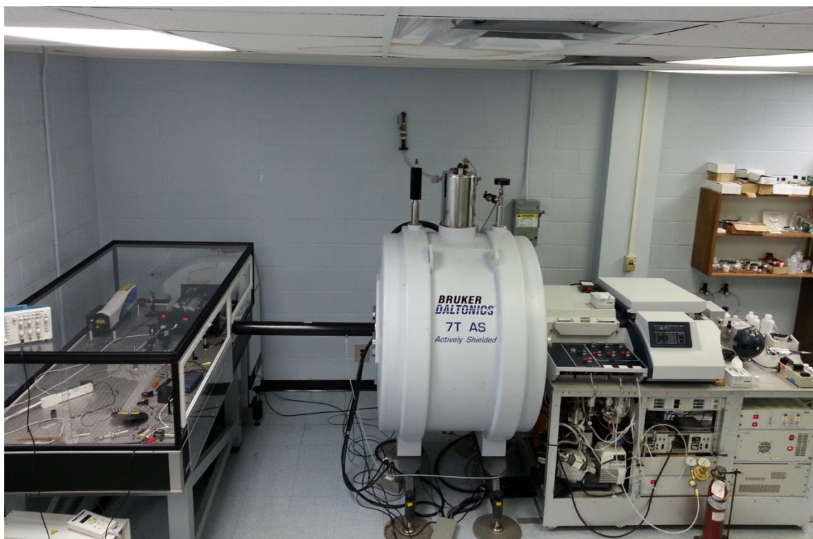
Figure 2.1. Photo of Bruker Apex-Qe7.0 T Fourier transform ion cyclotron mass spectrometer FT-ICR MS and a tabletop OPO laser at Memorial University.
