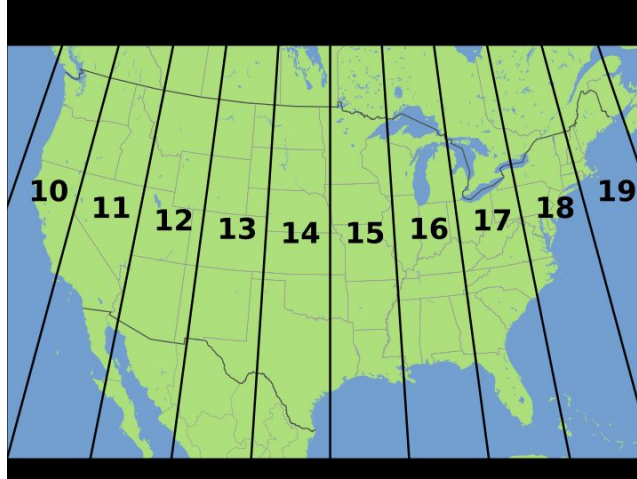
Figure 2.2: Visualization of UTM zones over the United States. Obtained under the Creative Commons License from the Wikimedia Commons.
