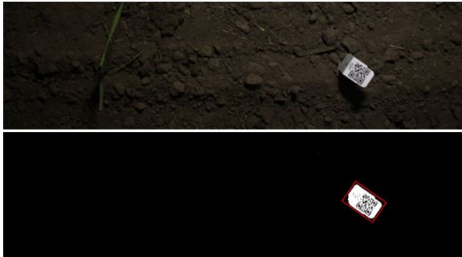
Figure 4.2: Binary image resulting from the HSV range filter. The overlaid red rectangle shows the rotated bounding box associated with QR code.
