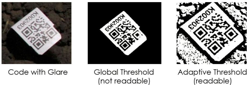
Figure 4.4: Comparison showing how an adaptive, rather than a global, threshold can make a code readable by keeping the bottom right corner intact.
