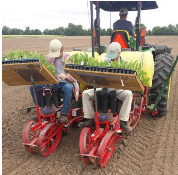
Figure 5.2: Two-row transplanter used for planting. Plants shown in the trays are a type of sunflower crop, not Kernza.
