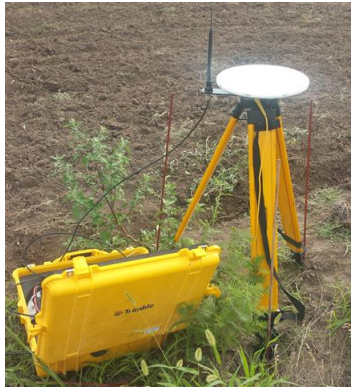
Figure 3.4: Ag542 base station mounted on tripod.
