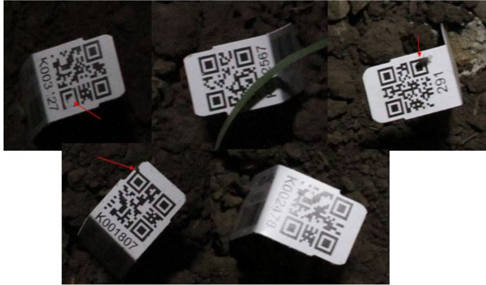
Figure 6.2: Unreadable codes. From left to right on top row: printer error, blocked by debris, blocked by fly. On bottom row: dirt, glare.
