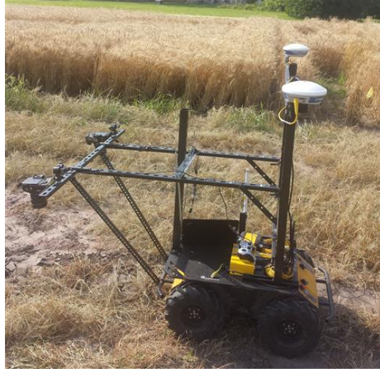
Figure 3.3: Husky mobile robot equipped with two cameras.
