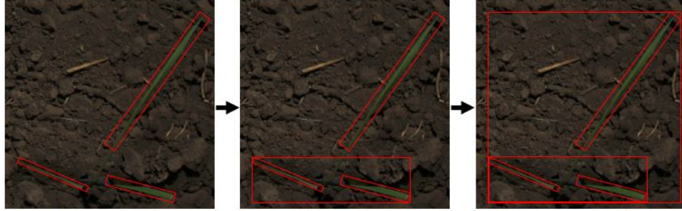
Figure 4.7: Example of hierarchical clustering. At each step the closest bounding boxes are merged together until there is one containing the entire plant.
