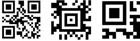
Figure 3.1: Comparison of 2D barcode formats encoding the text 1035 with high error correction. From left to right: Quick Response (QR), Aztec, and Micro QR.
