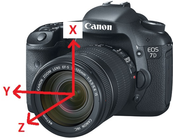
Figure 2.5: Image showing camera coordinate axes.
