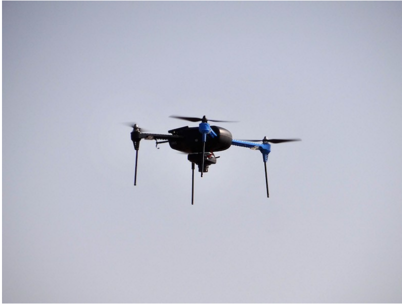
Figure 21 IRIS+ (3D Robotics, Inc, Berkeley, CA 94710, USA) a low cost UAV, carrying modified NIR Canon S100
