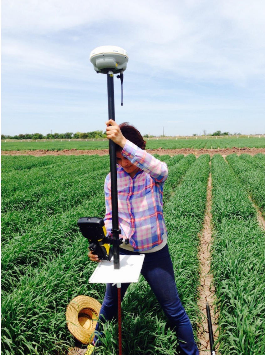
Figure 20 Surveying ground control points (GCPs) in the field using RTK GPS. Before the start of HTP 10-13 GCPs were uniformly distributed in the field.
